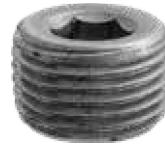
24255 Countersunk Thread: 1/2"-14 Length: 9/16"
