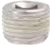
24217 Aluminum w/Sealant Square Countersunk Thread: 1/2"-14 Length: 9/16"
