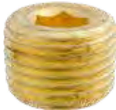
24249 Brass Countersunk Thread: 1/2"-14 Length: 9/16"
