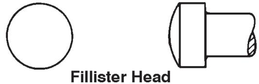
**Flat Fillister Head:** The flat fillister head has a flat top surface, cylindrical side surface and a flat bearing surface.
