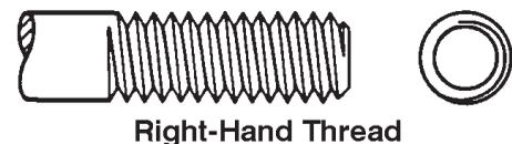
**Total Thread:** The total thread includes the complete or effective thread and the incomplete thread.
